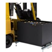
The optional FB/FTB battery roll-out feature allows easy replacement without a crane. Replacement time is significantly reduced.
