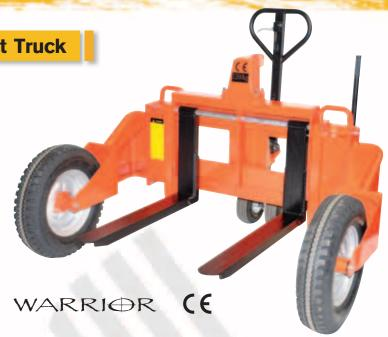
The new **WARRIOR** WRTT12 Rough Terrain Pallet Truck is ideal for outdoor applications where a conventional industrial truck just won't do! Mounted on large pneumatic tyred wheels all round, the truck just rides over undulating surfaces you find in some applications. With a capacity of 1200kg and an inside straddle width of 1277mm the WRTT12 will handle most pallets. Ideal for garden centers, building sites, farmyards and all other rough terrain applications.
